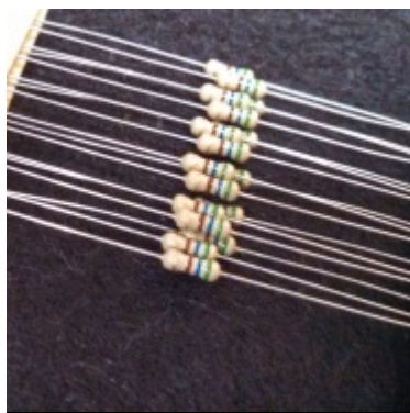
The stripes on a resistor help identify how much resistance is provided.
