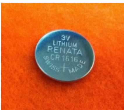
This is a "button" type battery. It provides 3 volts and this is the positive side.
