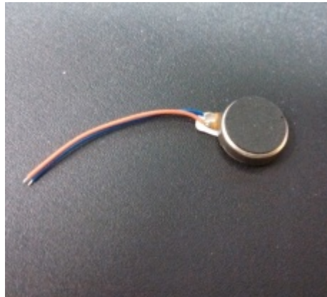
Cell phone vibrating motor. This motor is known as a "pancake" motor.
